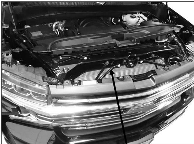
**(Fig 1) Remove cover and screws attaching grille**
